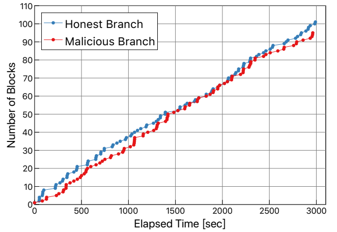
Fig. 6. The lengths of honest and malicious branches when v_m \sim U(1, 15) and the ratio of malicious nodes is 50%.
