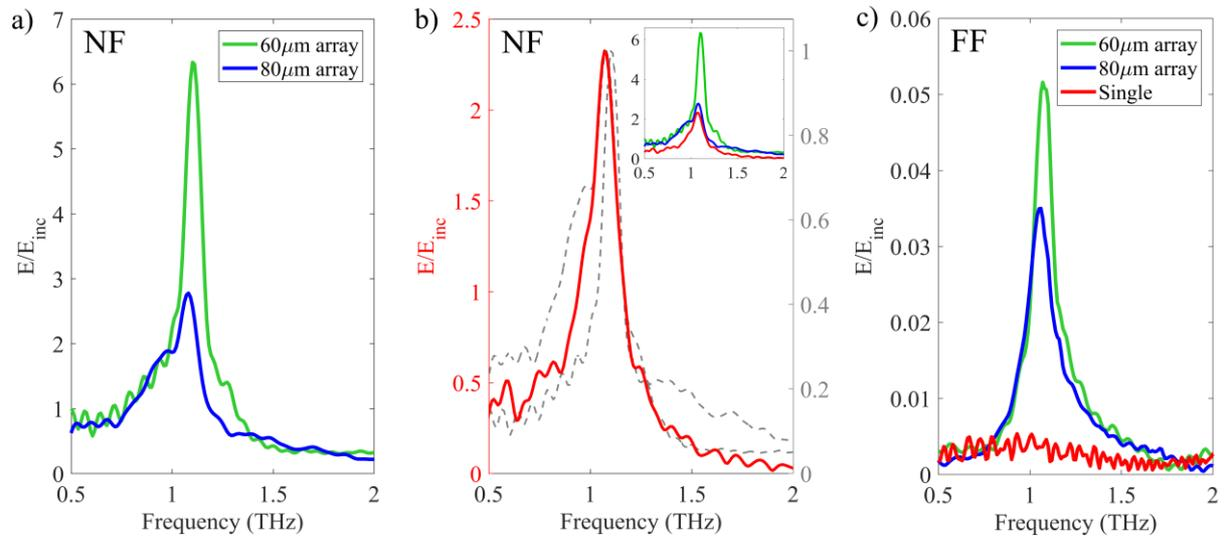
**Figure 3.** Simulation results: a) Simulated spectra in the far-field (interpolated) - measured transmission through face on the far end of the simulation region (shown in inset) b) Simulated near-field spectra measured using probe placed 1  $\mu\text{m}$  behind aperture (simulation region shown in inset).
