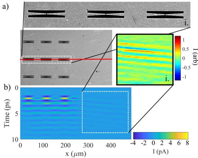
**Figure 5.** a) Interpolated near-field map of 80µm array b) Waveform recorded from 80 µm array showing time delay which the near-field map in (a) was recorded at, corresponding to the maximum amplitudes. c) Interpolated near-field map of single resonator at time corresponding to maximum of the waveform (inset).
