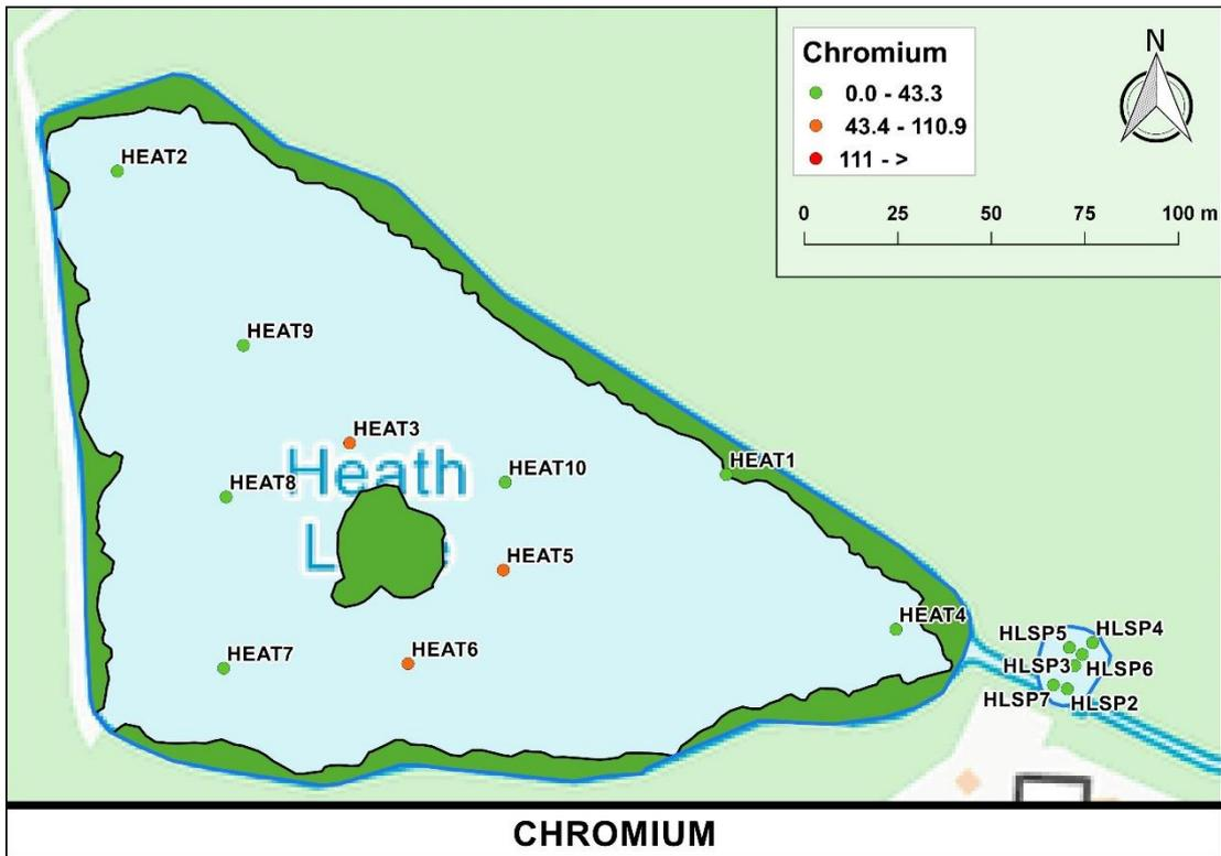
Figure 11 Distribution of chromium concentrations within Heath Lake and the sediment pond.
