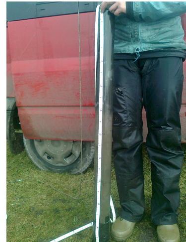
b Core MALH7, showing an upcore transition to more organic material at 42 cm depth
