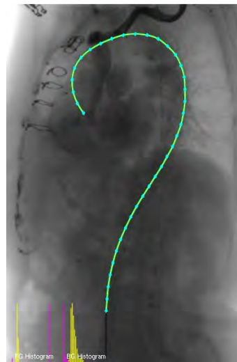
Fig. 4. Virtual reality simulation environment developed within CASCADE, used for rapid prototyping of novel catheters and algorithms. In the present view, sensor-based reconstruction of the catheter shape (green line) is evaluated by comparison with the simulated ground-truth (black/grey line). [left] fluoroscopy viewer - [right] 3D viewer of catheter in aorta.
