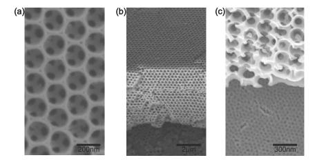
Figure 3. Scanning electron micrographs of the  $TiO_2$  double layer structure. (a) Top view of the (111) plane of the  $TiO_2$  inverse opal. (b) Cross-sectional view of the  $TiO_2$  double layer structure, with the inverse opal PC on top of a mesoporous layer. (c) Close-up view of the double layer interface, showing complete connectivity between the mesopores and the micropores.
