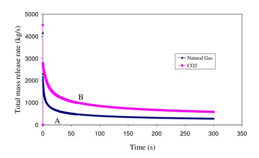
Figure 2. The variation of mass release rate with time following full bore pipeline rupture Curve A: Natural Gas (Piper Alpha) Curve B: CO2
