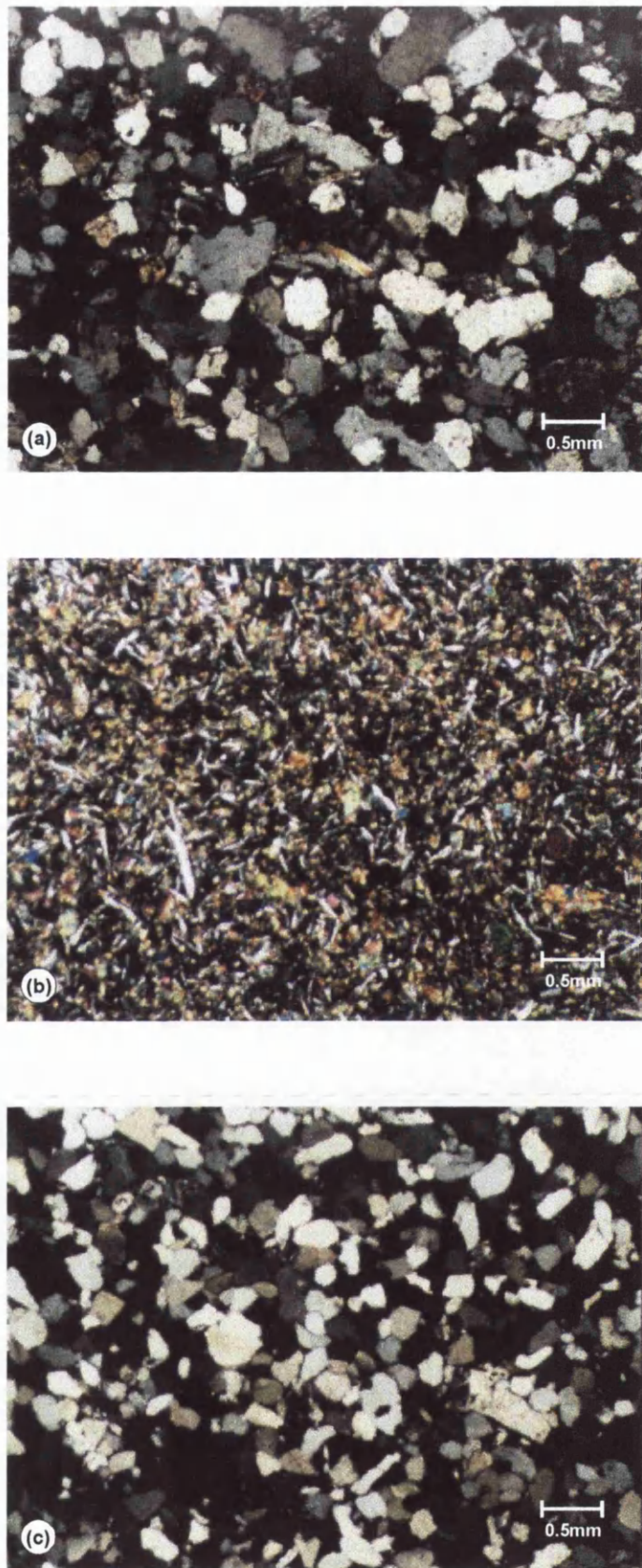
Figure 4-11 Photomicrographs of (a) Darley Dale sandstone, (b) Icelandic basalt and (c) Bentheim sandstone under cross-polarised light.
