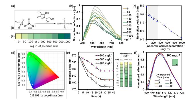
*Figure 5.* Characterization of the paper tear L-ascorbic acid sensor in the range between
