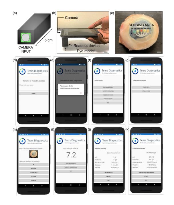
*Figure 8.* Smartphone readouts of contact lens sensors. (a) Schematic of the readout device; (b) Readout of a contact lens sensor exposed to artificial tear fluid on an ex vivo eye model; scale bar: 1.5 cm. (c) Photograph of the contact lens sensor inside the readout
