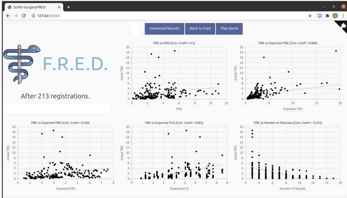
Figure 4: Results of 213 registrations using an anisotropic model of FLE
