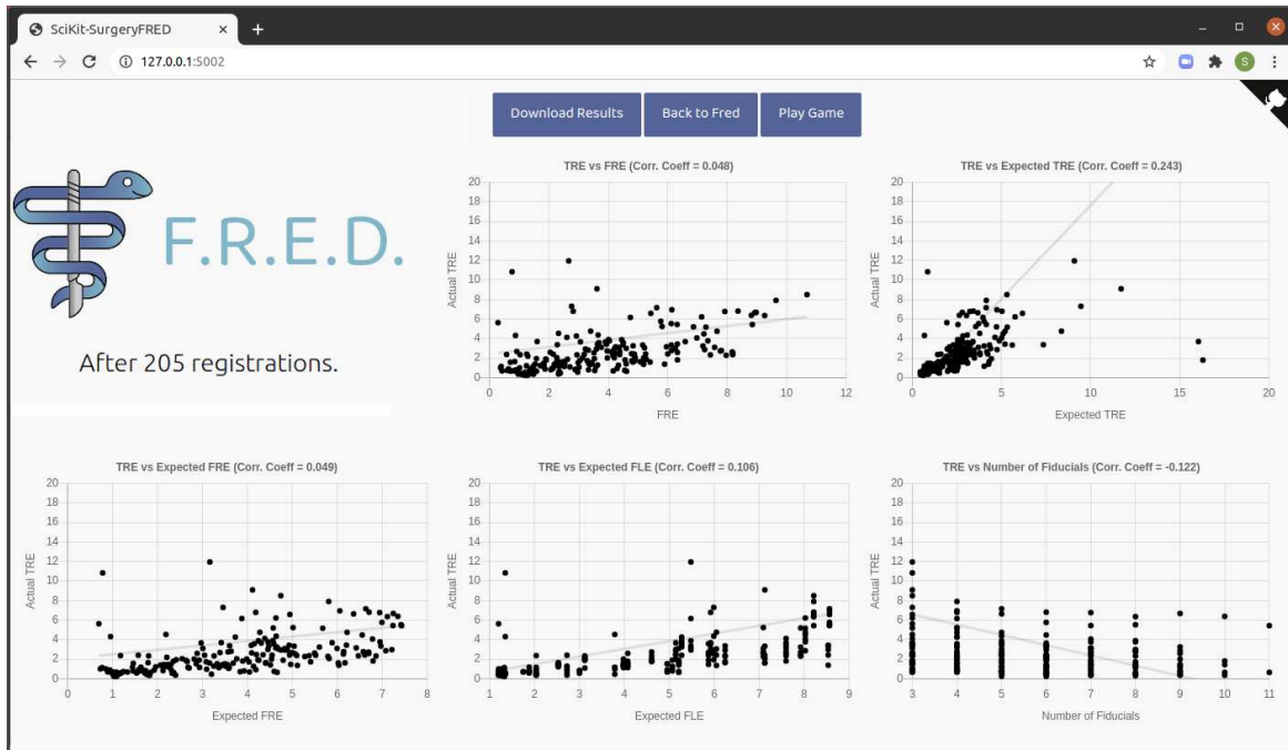
Figure 2: Plots of TRE against various error measures, generated by 205 user registrations.
