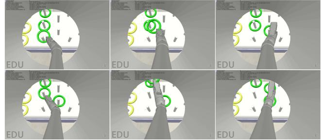
**Fig. 4:** The ring transfer task inside the CoppeliaSim simulation environment using the handle prototype.
