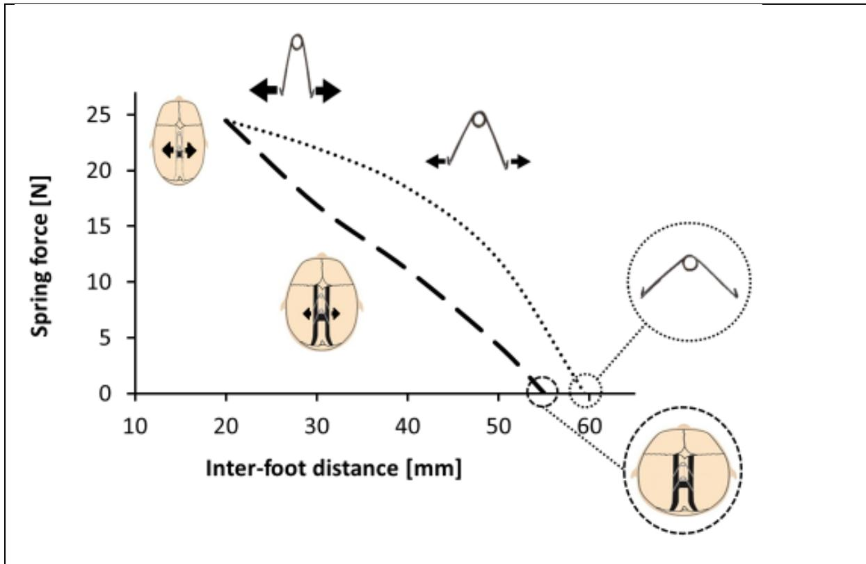
Figure 3: The graph shows in detail the stages of spring crimping and the forces exerted in this phase (top), compared to the forces exerted while inserted in the patient calvarium (bottom).
