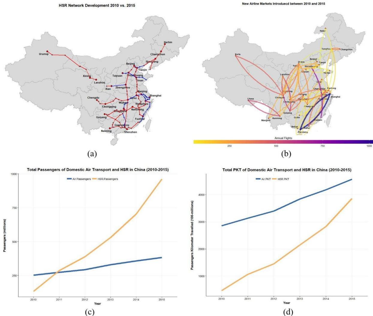
1 **FIGURE 1 Comparison between HSR and Domestic Air Transport networks 2010-2015.**
