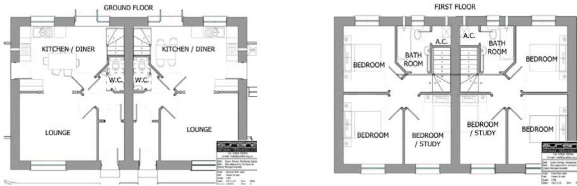
Figure 5: Pembroke Dock strawbale eco-houses: ground floor plan (left) and first floor plan (right)
