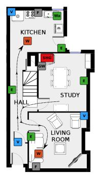
Figure 1: SPHERE device layout in the first floor of a residential house. SHG – the SPHERE Home Gateway. W – mobile wearables. V – video cameras with the attached video gateways. E – environmental sensors. Wa – the water sensor. F – forwarding gateways. GW – the main forwarding gateway attached to the SHG with a cable.
