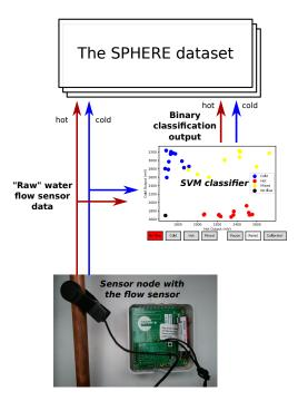
**Figure 11:** Overview of the water flow sensing subsystem [11]. A piezoelectric sensor is clamped on the water pipe, near the water tap; there is one clamp for the hot water pipe, and one for the cold one. The sensor data is delivered to the SPHERE Home Gateway, where the water flow status is classified with a machine learning algorithm. Both the raw flow values, the classification results, and the calibration data of the classifier are saved in the dataset.
