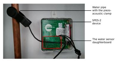
Figure 6: SPHERE Environmental Water Sensor.
