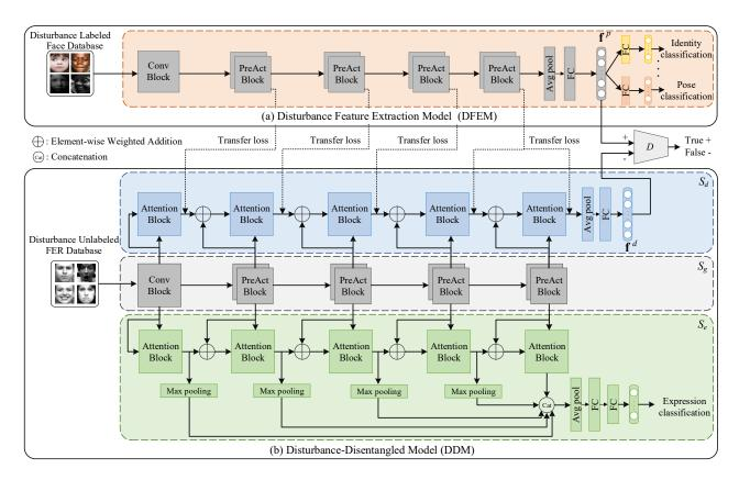
Figure 2: An overview of the proposed DDL method. DDL involves two stages. (a) Pre-training a DFEM consisting of the shared layers and the task-specific layers. The DFEM extracts features for identifying multiple disturbing factors. (b) Training a DDM consisting of a global shared sub-network  $(S_g)$ , an expression sub-network  $(S_e)$ , and a disturbance sub-network  $(S_d)$ . The DDM extracts expression-specific features by disentangling the disturbance information.
