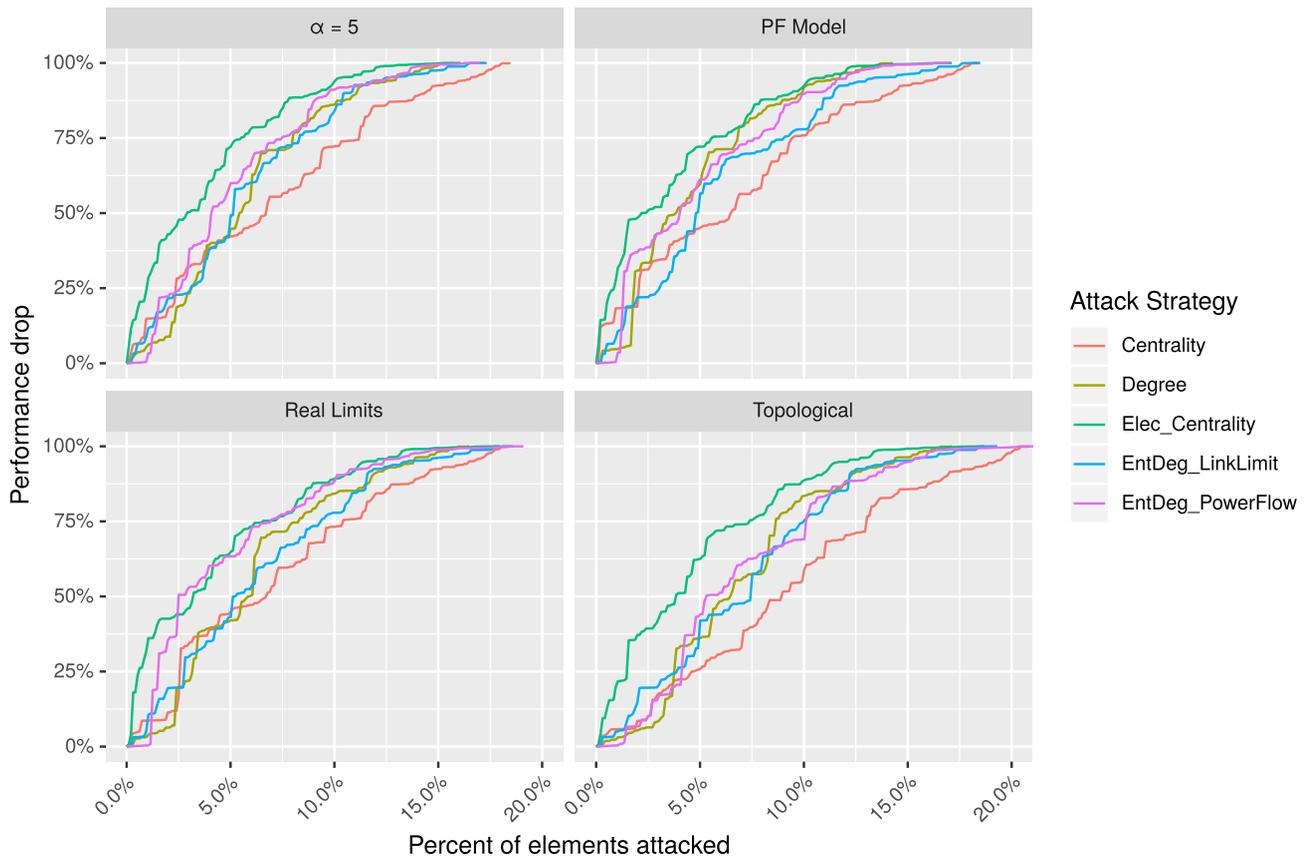
**FIG. 8.** The damage done to the power grid by each attack strategy by the percentage of the grid attacked. As can be seen, the strategy rank can change as a higher percentage of nodes is removed.
