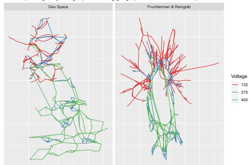
FIG. 2. UK power-grid voltage level shown in geographical space and graph space. The 132-V sections of the network are much less densely connected than the 275- and 400-V sections.
