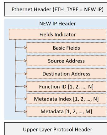
Fig. 1. NEW IP Header Structure.
