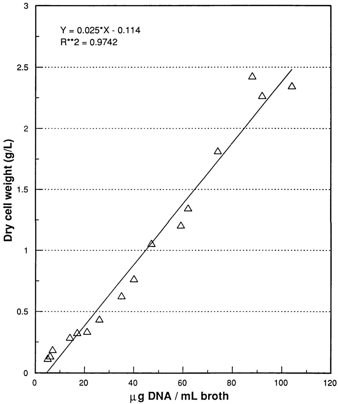
Figure 2.5 : Correlation of DNA content versus dry cell weight.
