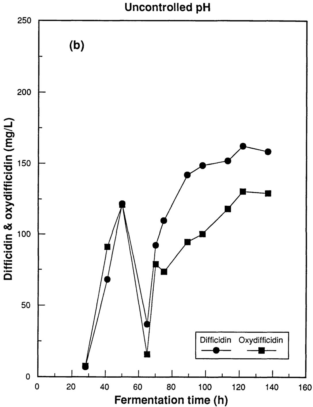
Figure 3.5: Continued (b) difficidin and oxydifficidin concentrations profiles.
