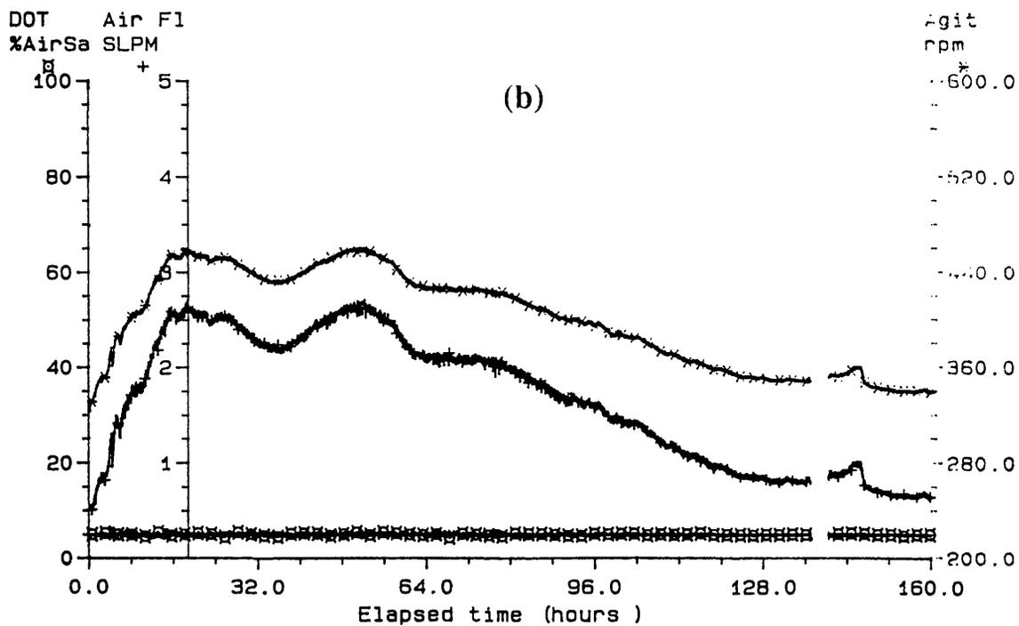
Figure 3.7 : Time profiles of an agitator speed, air flow rate and DOT at various controlled levels (a) 1% DOT (b) 5% DOT.
