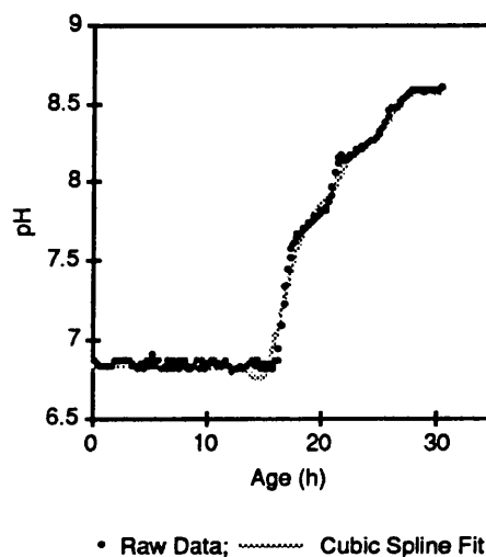
Figure A1.5: Cubic spline fits to pH data from fermentation batch C447. The user inputs were: relative error 0.01%, resolution 0.5, and goodness of fit 80%. The spline became oscillatory in an attempt to 'go around' the sharp corner. The fit was not acceptable.
