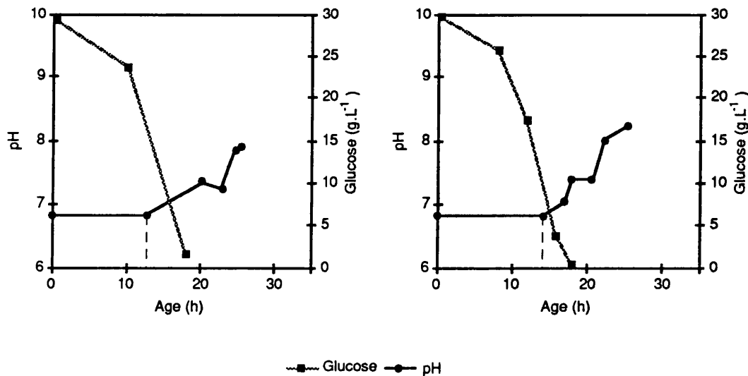
Figure 4.13: The end of pH control did not correspond with glucose exhaustion in batches C443 and C444 which underwent prolonged sterilisations. This implied that a nutrient, other than glucose, was limiting the growth. The availability of this essential nutrient had been reduced by the excessive heat stress.
