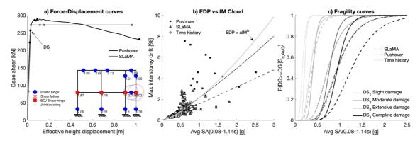
Figure 4: Transverse analysis results for the Pre-Code,  $L_{by}$ -4.5m,  $f_y$ -380MPa,  $f_c$ -24MPa building realisation.
