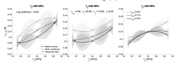
Figure 5: Pre-Code, transverse direction GP for the DS2 fragility median based on full time-history.
