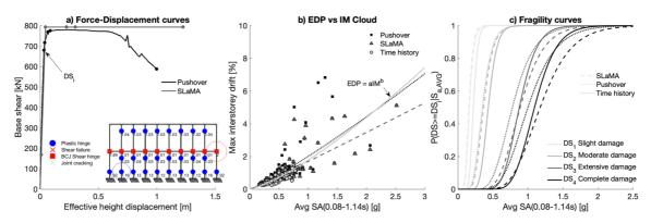
Figure 3: Longitudinal analysis results for the Low-Code, 9-bays,  $f_y$ -400MPa,  $f_c$ -19.7MPa building realisation.
