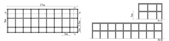
Figure 2: Geometry of the archetype building.
