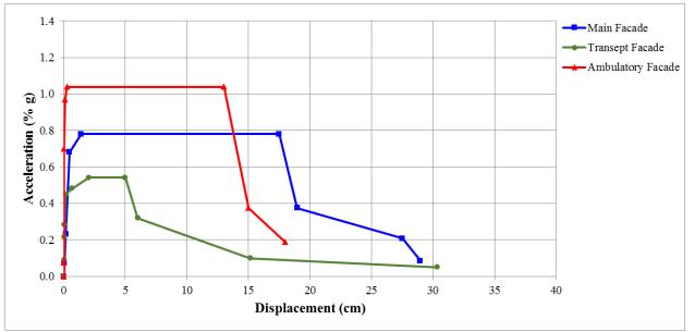
Figure 7. Macroelement capacity curves – Dimiao Complex
