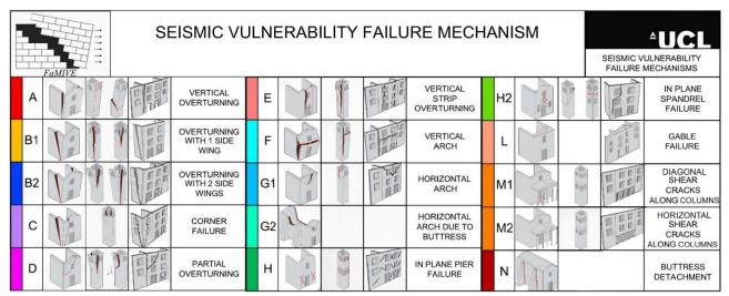
Figure 2. Suite of mechanisms analyzed by FaMIVE
