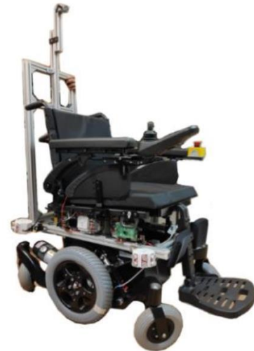
Figure 1. Our smart wheelchair with a collection of sensors
