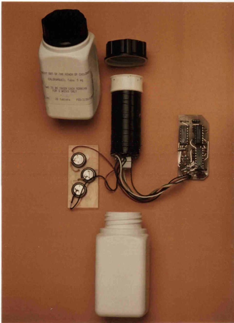
Figure 4.1 Photograph of the Electronic Recording Device and its Component Parts
