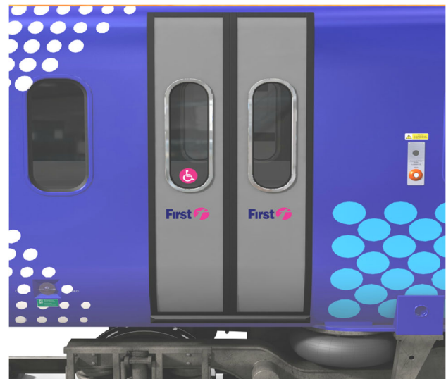
Fig. 5 The Class 380 train's passenger door unit
