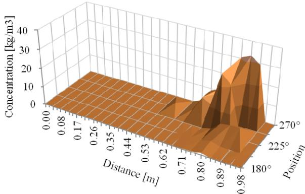
Figure 9: Local R290 concentration at wall unit discharge with 30 g/min and 480 m<sup>3</sup>/h airflow
