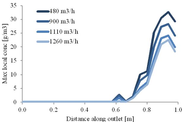
Figure 11: Maximum R290 concentration along discharge for different airflow rates
