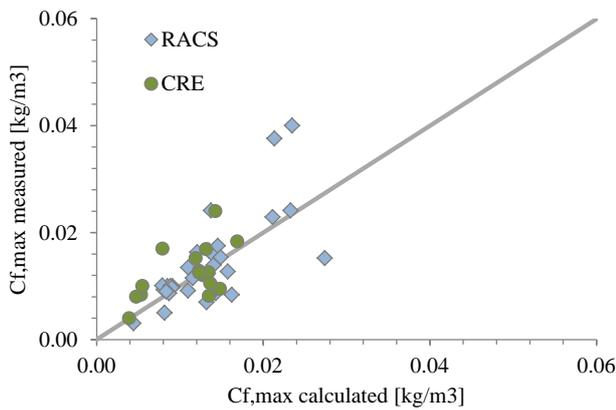
Figure 17: Comparison of measured maximum concentrations and unadjusted proposed formulae
