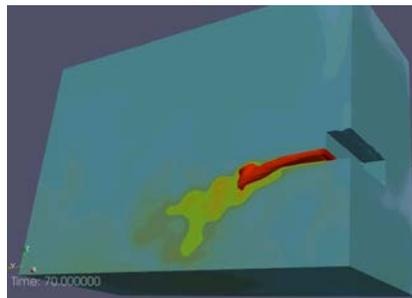
Figure 3: Contours\* showing trajectory,  $A_o = 0.05 \text{ m}^2$ , 500 g at  $141 \text{ g min}^{-1}$ ;  $x_T = 5.5 \text{ m}$ ; nearly all room air mixed within 70 s
