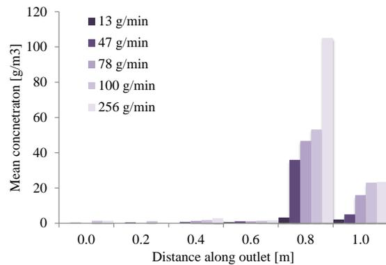
Figure 6: Measurements of R290 concentration within air discharged from an IDU at varying release mass flow rates
