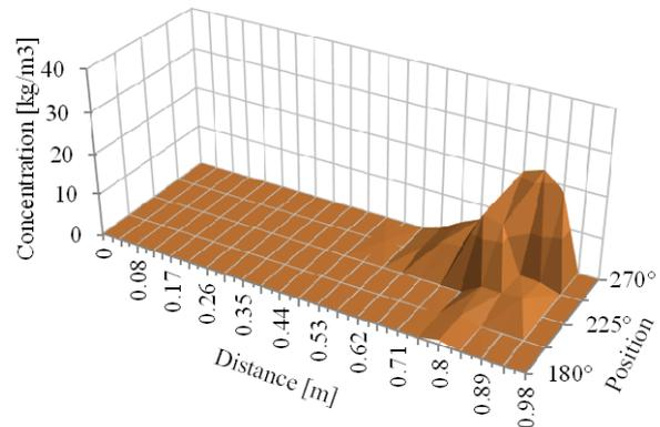
Figure 10: Local R290 concentration at wall unit discharge with 30 g/min and 1260 m<sup>3</sup>/h airflow
