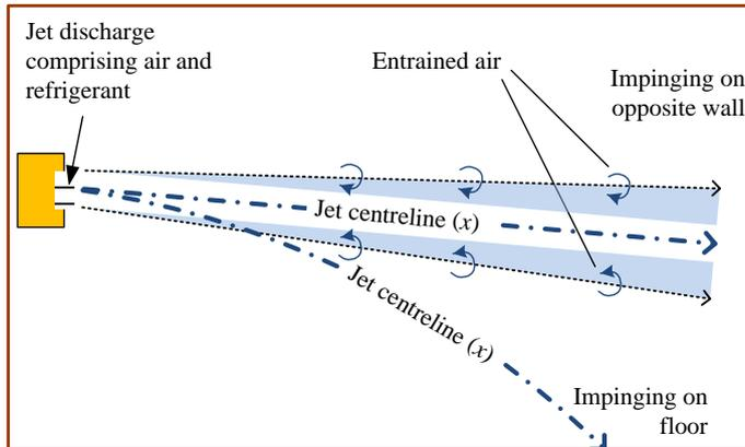
Figure 1: Schematic of entrainment process and jet termination
