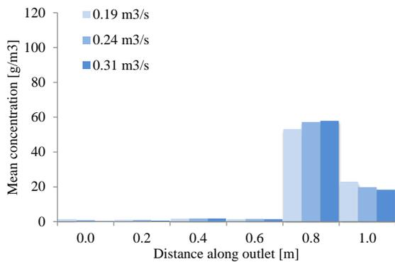
Figure 5: Measurements of R290 concentration within air discharged from an IDU at varying airflow rates
