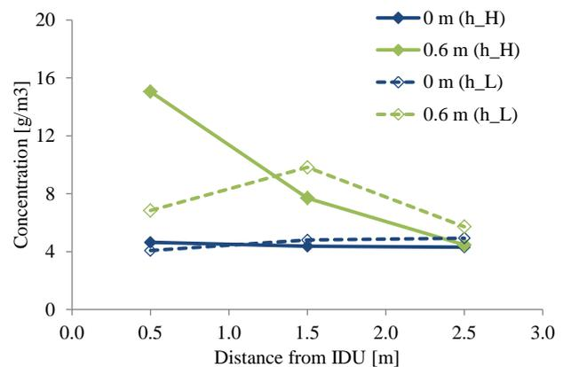
Figure 16: Local concentrations in front on air discharge; 480 m<sup>3</sup> h<sup>-1</sup>, 120 g min<sup>-1</sup> and 200 g
