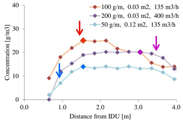
Figure 14: Floor concentrations during a release (g/min) within the IDU with outlet opening (m<sup>2</sup>) and airflow (m<sup>3</sup> h<sup>-1</sup>) at different conditions
