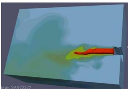
Figure 2: Contours\* showing trajectory,  $A_o = 0.20 \text{ m}^2$ , 500 g at  $141 \text{ g min}^{-1}$ ;  $x_T = 5.5 \text{ m}$
