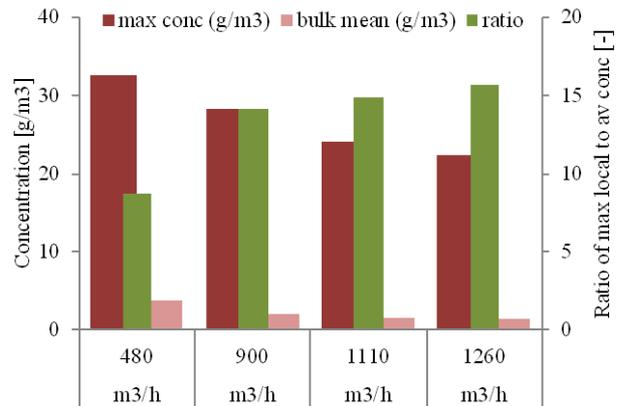
Figure 12: Comparison of maximum concentration and bulk mean concentration
