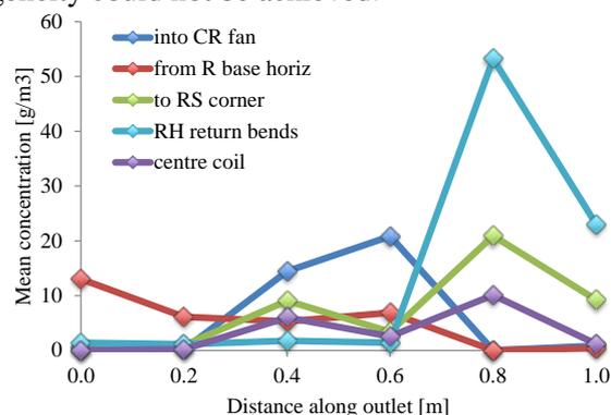
Figure 8: Average concentration at linear distances along air discharge arising from different release points
