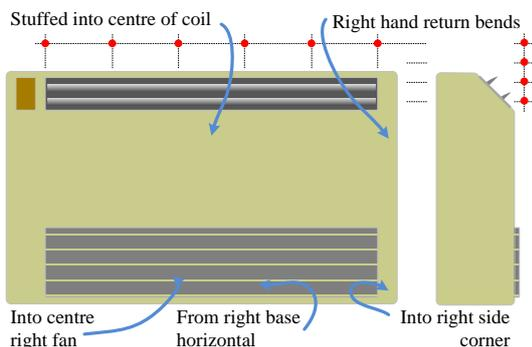
Figure 7: Positions/direction of additional release points and position of sampling points (red dots)
