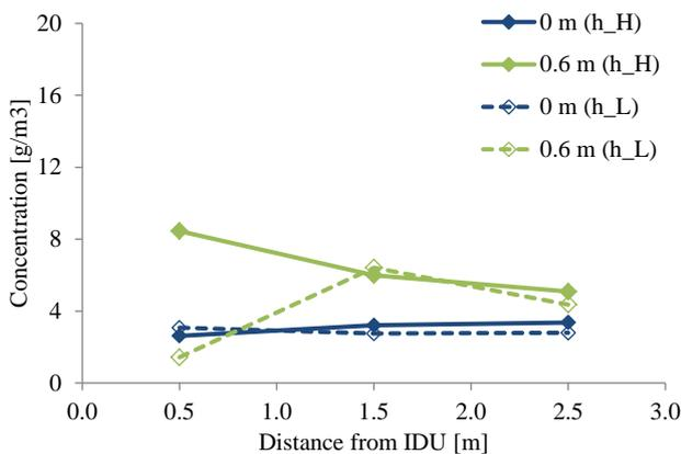
Figure 15: Local concentrations in front on air discharge; 1260 m<sup>3</sup> h<sup>-1</sup>, 120 g min<sup>-1</sup> and 200 g
