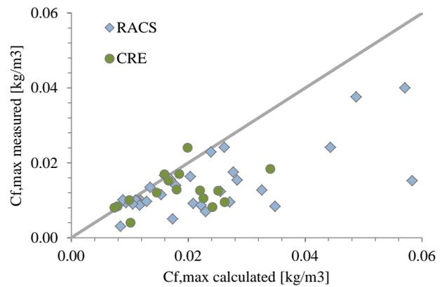
Figure 18: Comparison of measured maximum concentrations and proposed formulae adjusted to "catch all"
