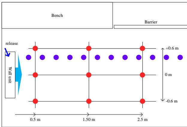
Figure 13: Layout of test room (3.5 m × 4 m) with sampling points indicated
