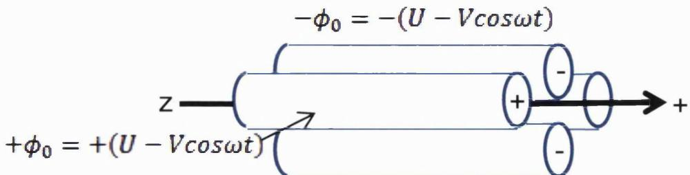
Figure 1.4: Schematic of a quadrupole. RF and DC voltages applied along x and y axis changing to scan across the field and allowing only ions with stable trajectories in the scanned region to pass through.  $\Phi_0$  represents the potential applied to the rods,  $\omega$  is the angular frequency (rad/s =  $2\pi\nu$  where  $\nu$  is the frequency of the radio frequency, U is the direct current and V is the RF amplitude. Modified from Lane, C 2005.<sup>13</sup>
