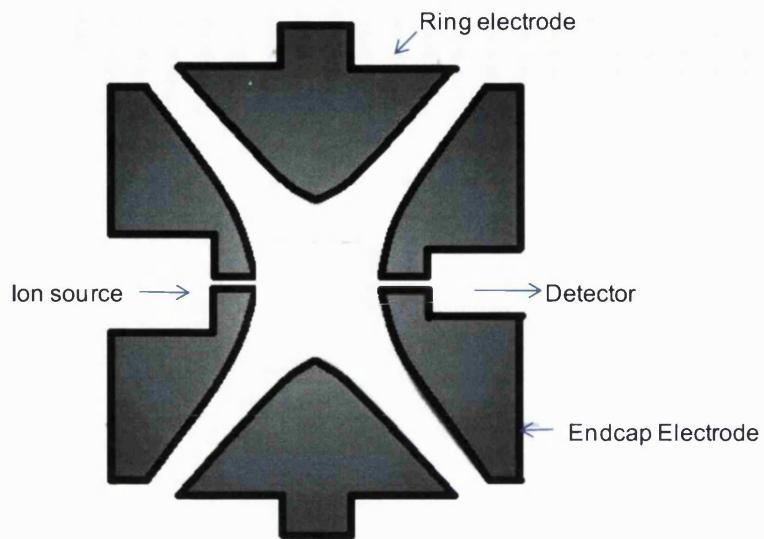
**Figure 1.5: Schematic representation of an iontrap.** Ring electrodes and endcap electrodes maintain ions of certain  $m/z$  in the trap for analysis and allow all others to be ejected to the detector. Selected ions can then be fragmented to acquire MS/MS data or  $MS^n$  data.
