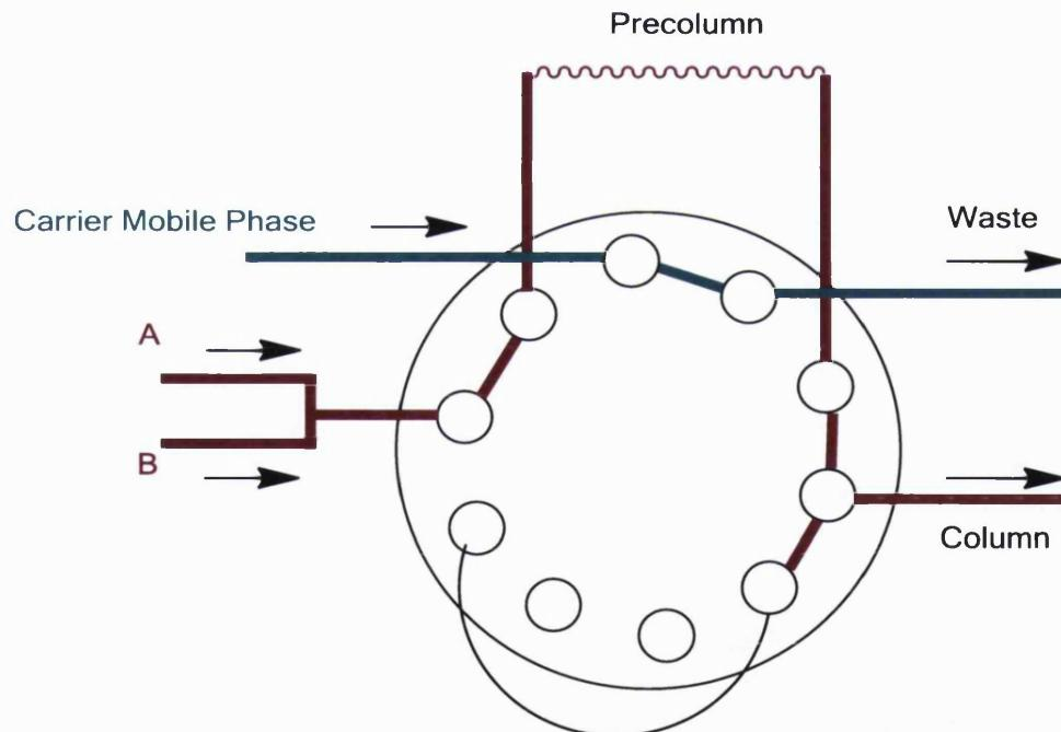
**Figure 4.2: Stream Select Switching Valves.** A) shows the valves in the initial position where the flow from the carrier mobile phase goes through the pre-column and goes to waste to desalt. After three minutes, the stream select valve switches over to B) and the flow from both A and B are mixed together and go through the pre-column and into the column to be finally eluted into the mass spectrometer.
