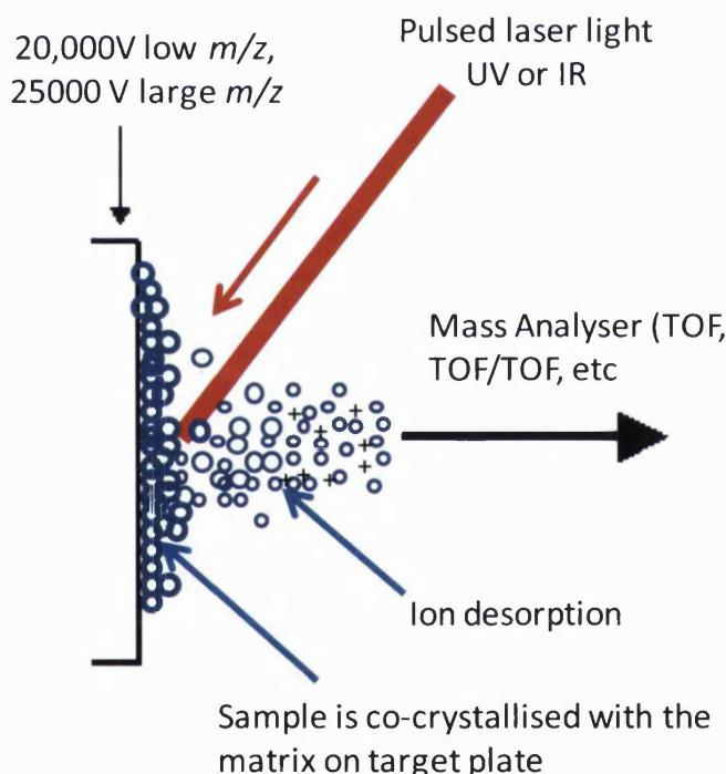
**Figure 1.3: Desorption and ionisation of sample from a MALDI target plate.** The mixture of matrix and sample are spotted onto a target plate and allowed to dry before being ablated by a laser of UV or IR wavelength which the matrix is able to absorb. The matrix and sample are desorbed and ionised in a plume as they leave the plate and enter the mass analyzer.
