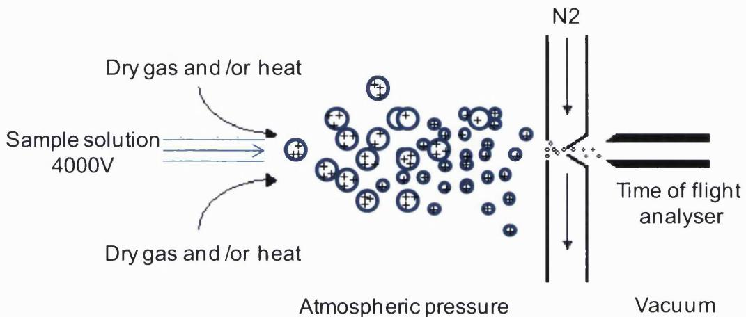
**Figure 1.2: Example of the ionisation process on the tip of an electrospray ion source. A positive charge is applied to the capillary which results in positively charged ions to be dispersed from the tip. These migrate away from the capillary as small droplets which are reduced to size and eventually disappear leaving only the ionised analyte. Image modified from Lane, 2005.<sup>13</sup>**
