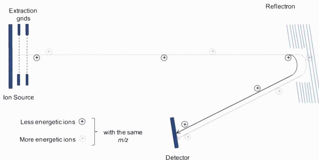
**Figure 1.6: Schematic of a time-of-flight reflectron mass analyser. Samples travel through the flight tube, spreading out to be focused in the reflectron before reaching the detector. Modified from Lane, C, 2005.<sup>13</sup>**
