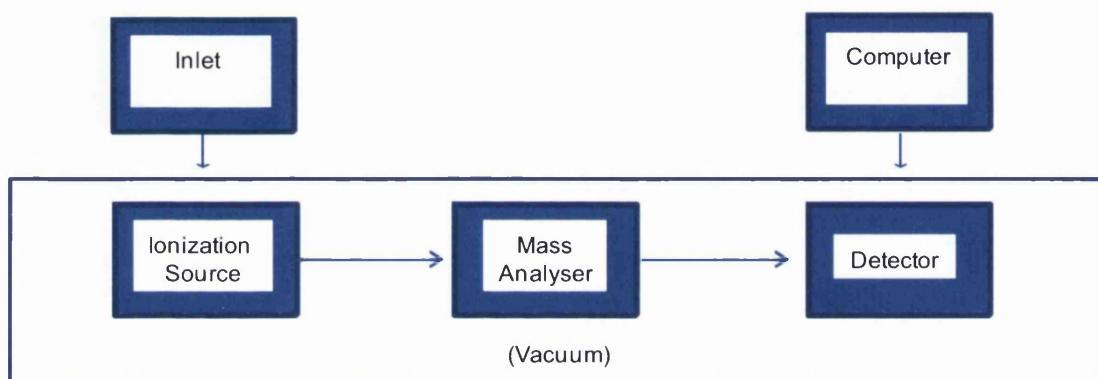
**Figure 1.1: The components of a mass spectrometer**
