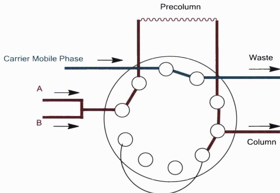
Figure 3.5: Stream Select Switching Valves. (A) shows the valves in the initial position where the flow from the carrier mobile phase goes through the pre-column and goes to waste to desalt. After three minutes, the stream select valve switches over (B) and the flow from both A and B are mixed together and go through the pre-column and into the column to be finally eluted into the mass spectrometer.
