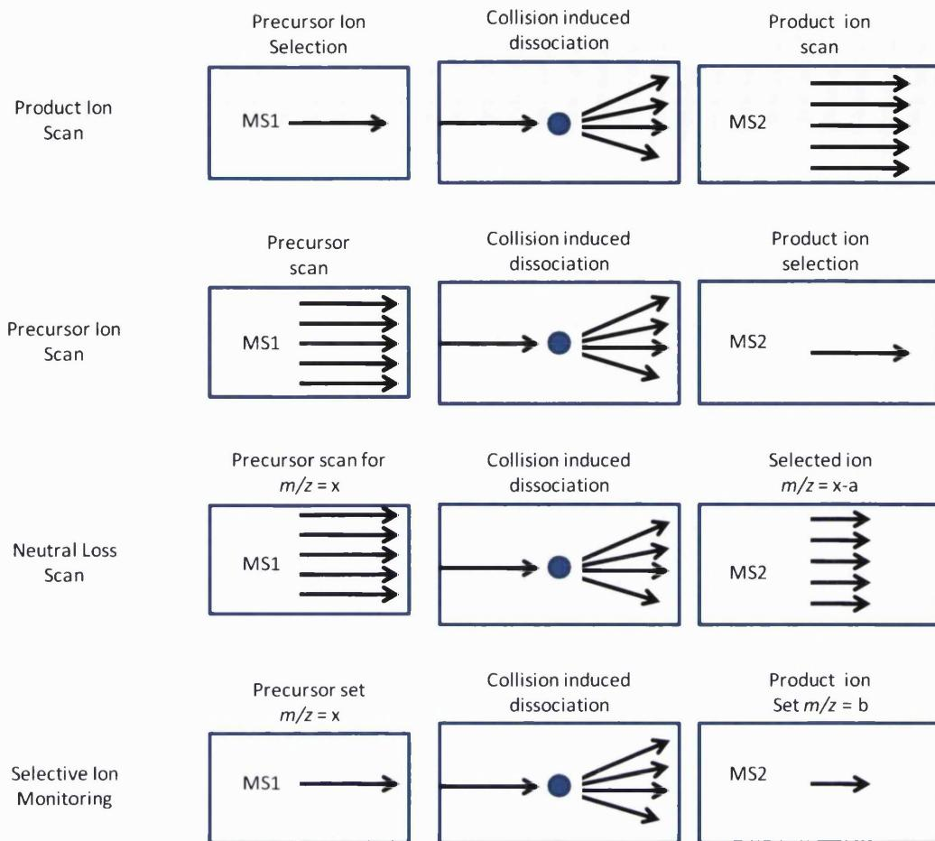
**Figure 1.7: Four types of tandem analysis experiments that can be performed using a triple quadrupole.**
