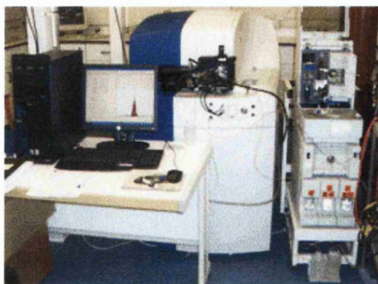
Figure 42 Micromass Q-TOP Global Tandem Mass Spectrometer (Photo and instrument specifications from www.pharmacy.ac.uk )
