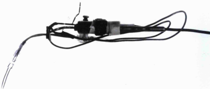
Plate 2.2 Photograph showing recording electrode used for both carotid chemoreceptor fibre and phrenic nerve recordings. The electrode comprises a Neurolog headstage (NL100AK), with stainless steel recording hooks, and an earthing lead.
