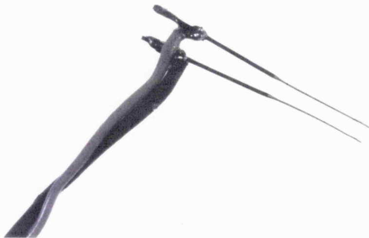
Plate 3.1 Photograph showing custom-made stimulating electrode for somatophrenic experiments. The bipolar hooks were dental brooch needles; the teeth on these needles proved particularly effective for maintaining a good contact with the sciatic/median nerves.
