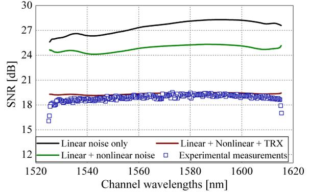
Fig.2: Signal-to-noise ratio including different noise components versus wavelength after 630 km [11].
