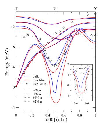
FIG. 6. (Color online) Theoretical results using the same calculations as reported in Ref. [8]. The experimental points at room temperature for key modes are shown—see Ref. [7]. The  $\alpha$ -U structure is unstable at T = 0 K as shown by the soft phonon at h = 0.5 having an imaginary frequency. The inset shows how this frequency changes as  $a_U$  is either compressed or expanded. The thin film refers to U/W.
