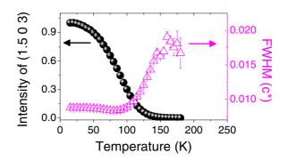
FIG. 5. (Color online) The integrated intensity of the  $(1.5 \ 0 \ 3)$  CDW reflection as a function of temperature for the 1500 Å film is represented by the solid black points and the left-hand y-axis scale. The width of the  $(1.5 \ 0 \ 3)$  reflection is represented by the open magenta triangles and the right-hand y-axis scale.
