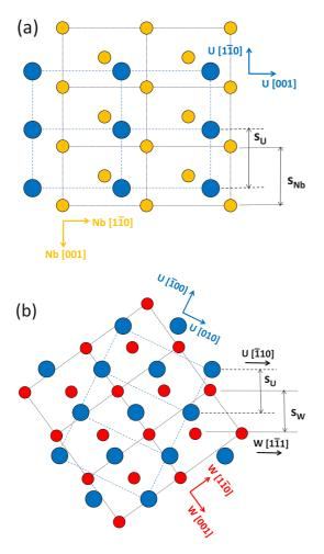
FIG. 1. (Color online) Epitaxial relationship for  $\alpha$ -U (blue circles) on (a) Nb ( $a_0 = 3.300$  Å) and (b) on W ( $a_0 = 3.165$  Å). For the (a) orientation the governing factor is the distance in the horizontal plane between rows of U atoms,  $s_U = \frac{1}{2}(a_U^2 + b_U^2)^{\frac{1}{2}} = 3.264$  Å. For the orientation (b), the rows of U and W atoms must be within register so it is necessary that the uranium  $s_U = d(110)_U$  must be close to the tungsten  $s_W = 2d(112)_W$ .
