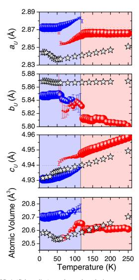
FIG. 4. (Color online)  $a_U$ ,  $b_U$ , and  $c_U$  lattice parameters, and the atomic volume as a function of temperature for the U/W film of 1500 Å. The open stars give the bulk values [15]. The red points represent the high-temperature phase and the blue, the low temperature phase, in which the CDW appears. The size of the points is an indication of the volume of the sample that has such a lattice parameter.
