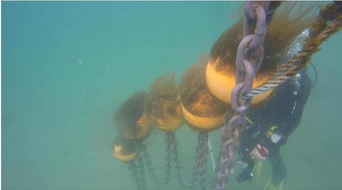
**Figure 7.** Float system attached to helical anchor on an ecologically friendly mooring trial in Torbay Harbour. Photo credit: Mark Parry CSI.
