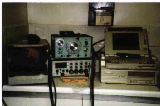
Figure A3d: The ERG recording machine. From left, monitor connected to the infra-red camera within the ganzfeld to monitor the position and condition of the subject, the Grass stimulator and amplifier, and the PC based data acquisition system
