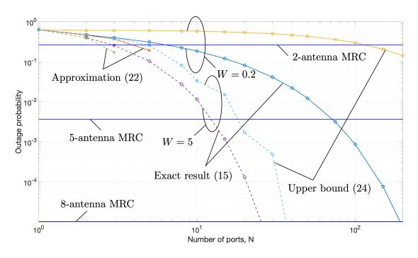
Figure 4: Outage probability approximations and bounds for the FAS when  $\frac{\gamma_{\text{th}}}{\Gamma} = 0 \text{dB}$ .
