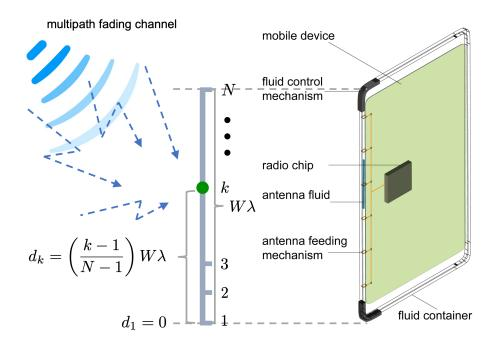
Figure 2: A possible architecture for a FAS.
