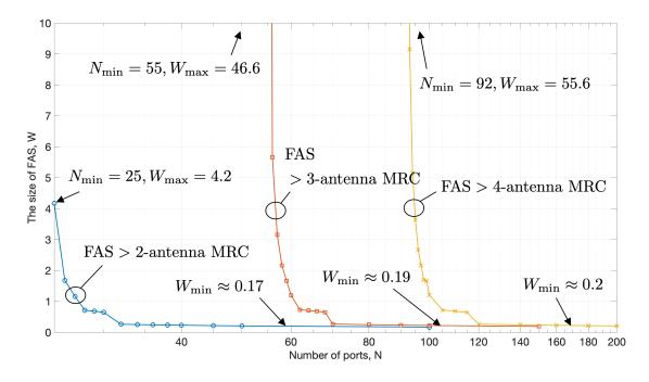
Figure 5: The required size of the FAS based on (29) for outperforming the respective MRC system when  $\frac{\gamma_{\text{th}}}{\Gamma} = 0 \text{dB}$ . For example, 'FAS>2-antenna MRC' means that FAS outperforms 2-antenna MRC.
