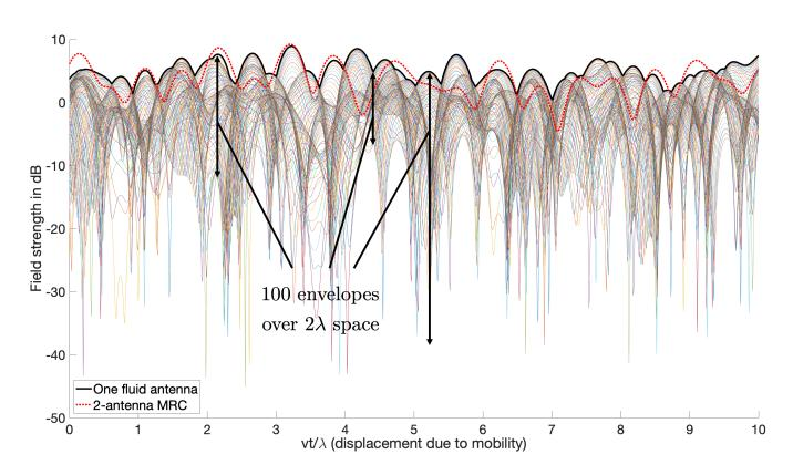
(b) Comparison for a 100-port FAS with  $2\lambda$  space and MRC at 5GHz at  $v=30\mathrm{km/h}$
