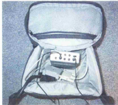
Figure G.3: The psychophysiological monitoring equipment was placed inside a wearable pack for the participant's comfort. This also ensured that the delicate optical cable remained protected, minimising signal failures.
