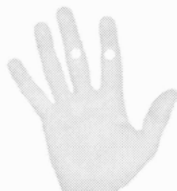
Figure G.2: The bipolar EDA sensors were attached as illustrated to the index and middle fingers of the participant's non-dominant hand.
