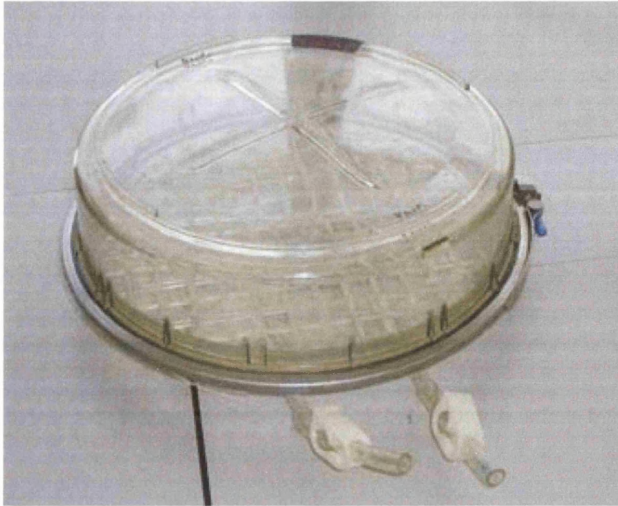
Figure 2.1 The Billups Rothenburg Chamber™, used for the culture of cells under hypoxic conditions.
