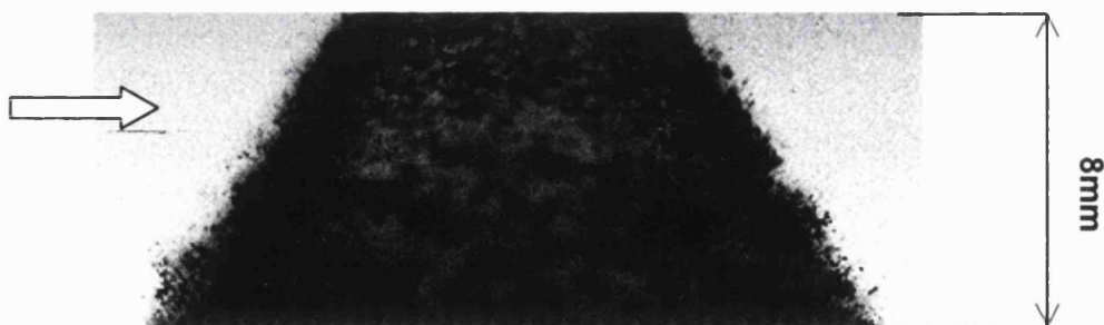
Figure 2.13 - Injector A: atmospheric pressure, 23°C fuel temperature, 55 bar fuel pressure, gasoline, 1.6 ms aSOI, figure A1.1 062.
