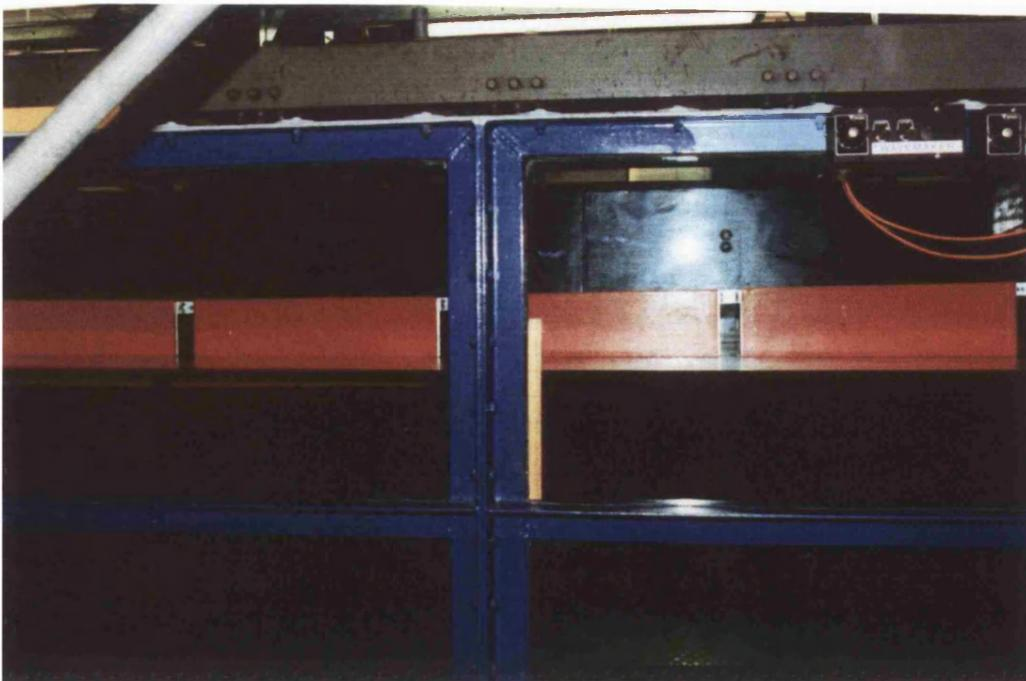
Figure 5.9 Load applied on pontoon module 3 in single array with Hinged-Rigid connection
