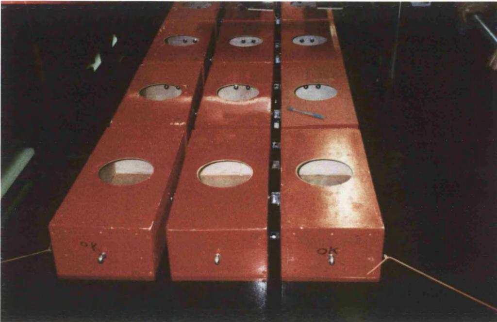
Figure 5.6 Assembly pontoons for hinged connection for mat array
