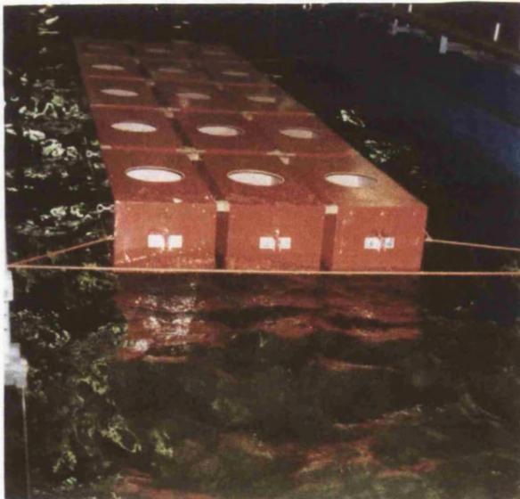
Figure 5.14 Mat array of pontoons with Hinged-Rigid connection in wave
