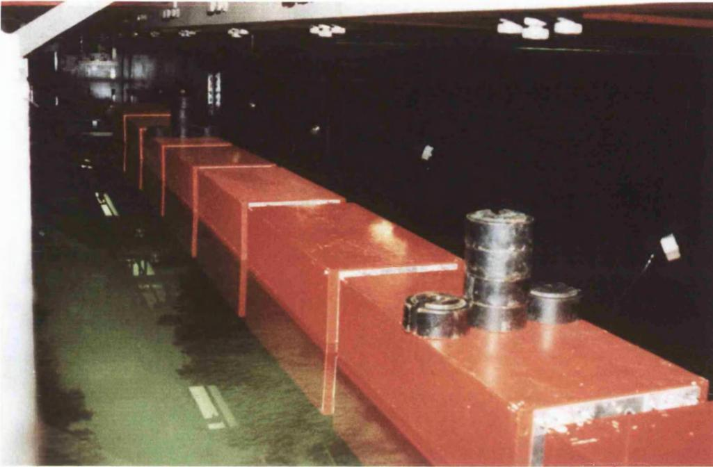
Figure 5.8 Load applied on pontoons module 3 and 7 in single array
