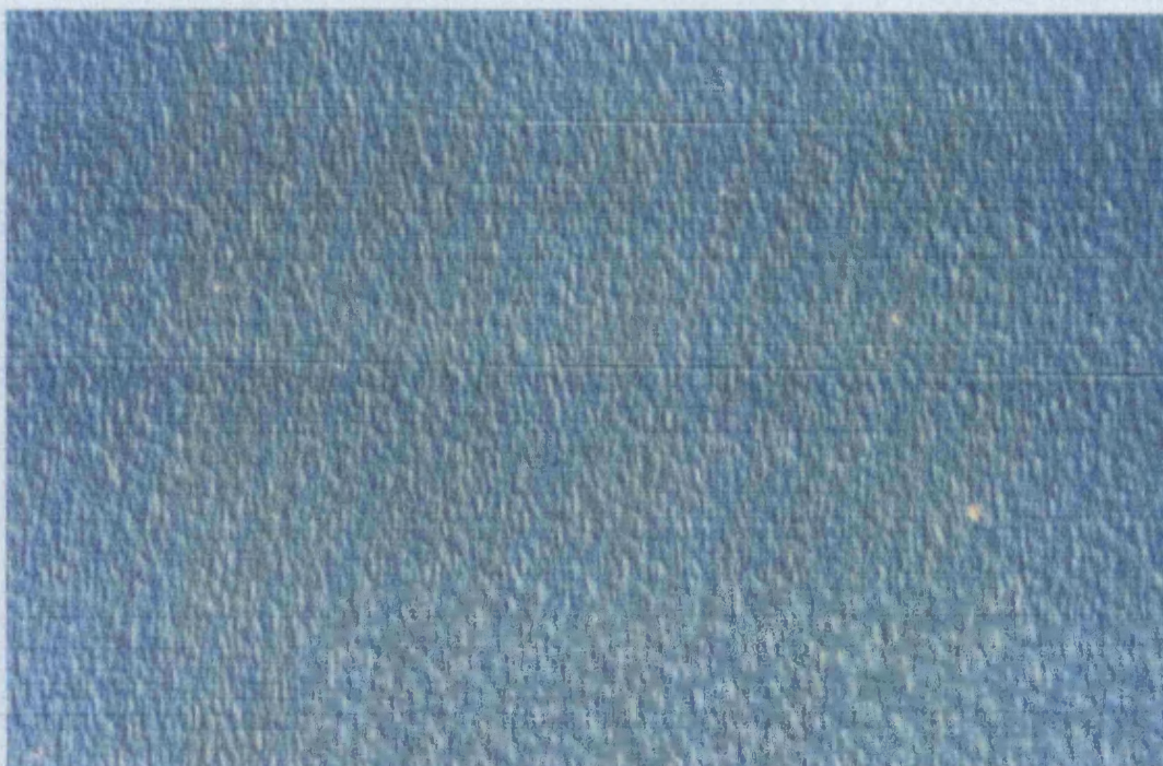
Figure 3.18b Nomarski optical micrograph of the M199 reflector stack, grown on silicon by MBE. The magnification and surface area are as above. A slightly coarser texture can be observed, and this is believed to be responsible for the lower reflectivity measured on this wafer (Chapter 5).
