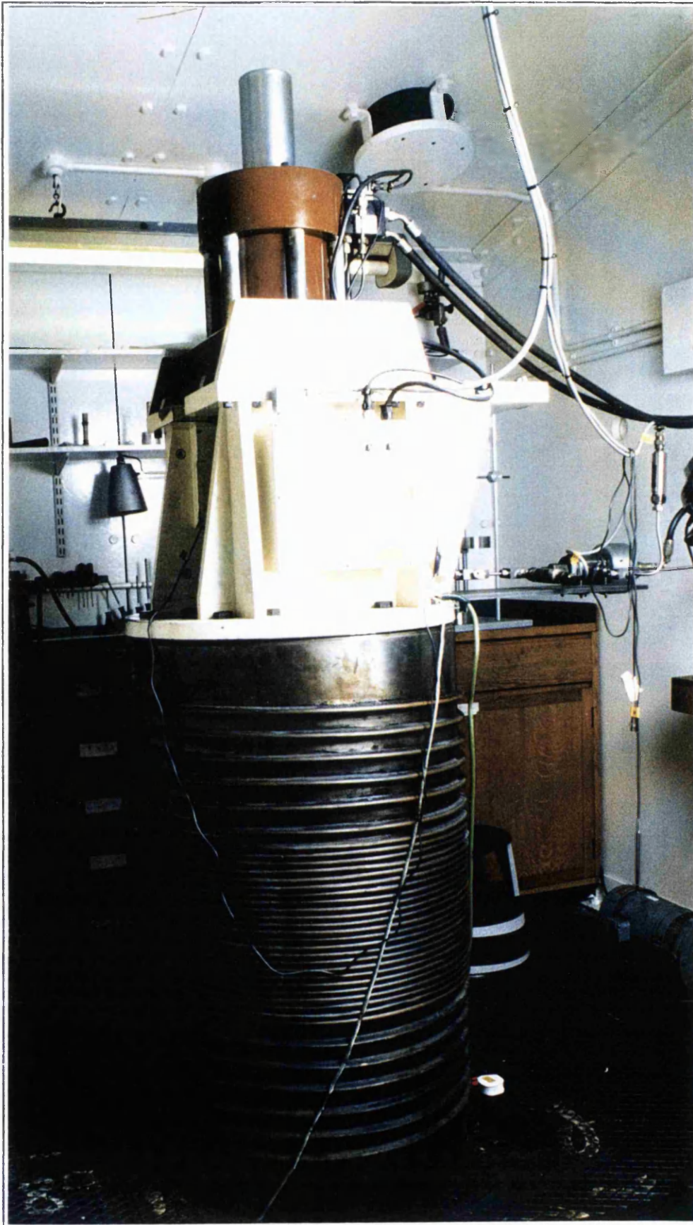
Fig. 4.1.a. Photograph of the high pressure triaxial deformation vessel (modified).
