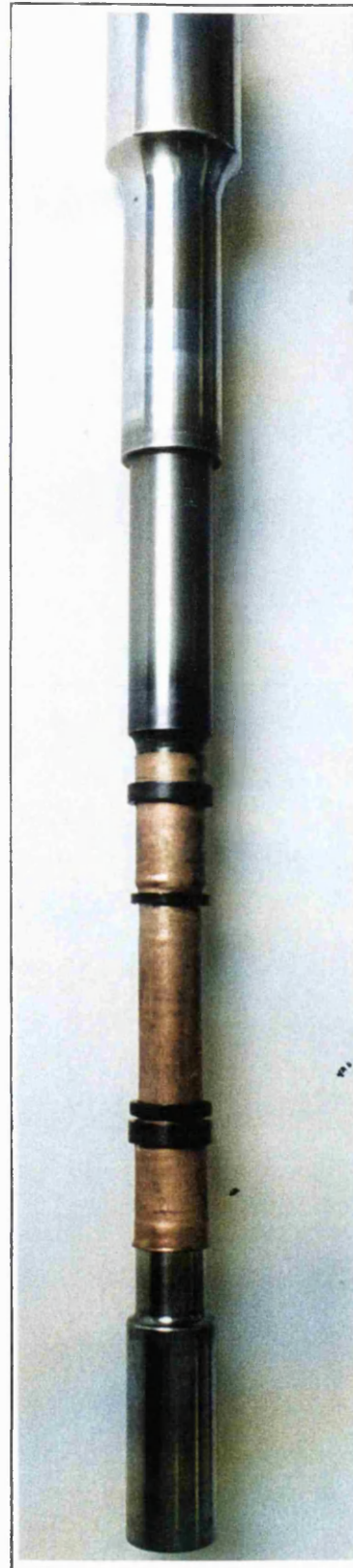
Fig. 5.2.1.1.a. Photograph of piston/specimen/lower ram assembly showing jacket and sealing rings.
