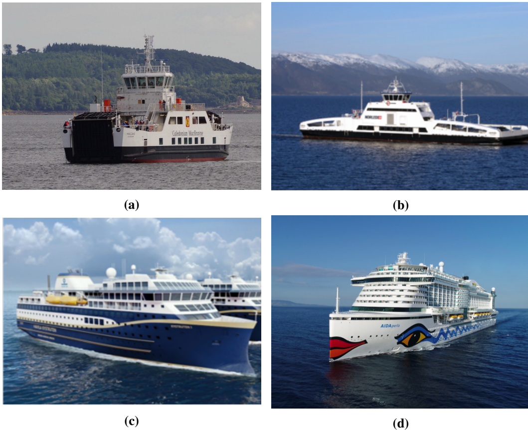
Figure 2.12: Battery-powered ships. (a) hybrid diesel-battery Caledonian MacBrayne ferry MV Hallaig ((Geertsma et al., 2017)). (b) Norwegian all-electric battery-powered ferry MF Ampere (Alnes et al., 2017). (c) Havila Kystruten 's hybrid gas-battery ship (Corvus, 2019a). (d) World's largest battery maritime application: 10 MWh with LNG engines (Corvus, 2019b).
