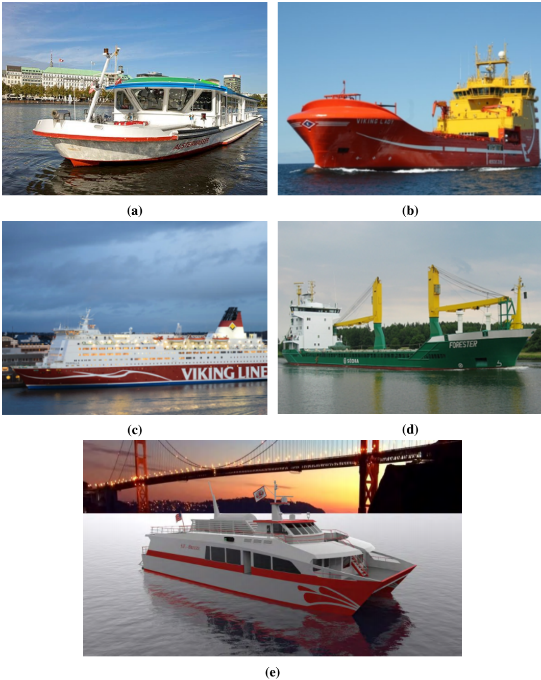
Figure 2.7: Fuel cell powered ships. (a) FCS Alsterwasser with 96 kW PEMFC (McConnell, 2010). (b) FellowSHIP with 320 kW MCFC (Ovrum and Dimopoulos, 2012). (c) MS Mariella with 60 kW HT-PEMFC (Tronstad et al., 2017). (d) MS Forester with 100 kW SOFC (Tronstad et al., 2017). (e) SF-BREEZE with 4920 kW PEMFC (Pratt and Klebanoff, 2016).
