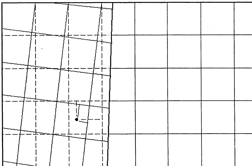
Figure 3.2 The solution to the problem of the two UTM zones in the Guadalquivir Valley, showing how the coordinates of the same point can be shifted from one system of reference to another
