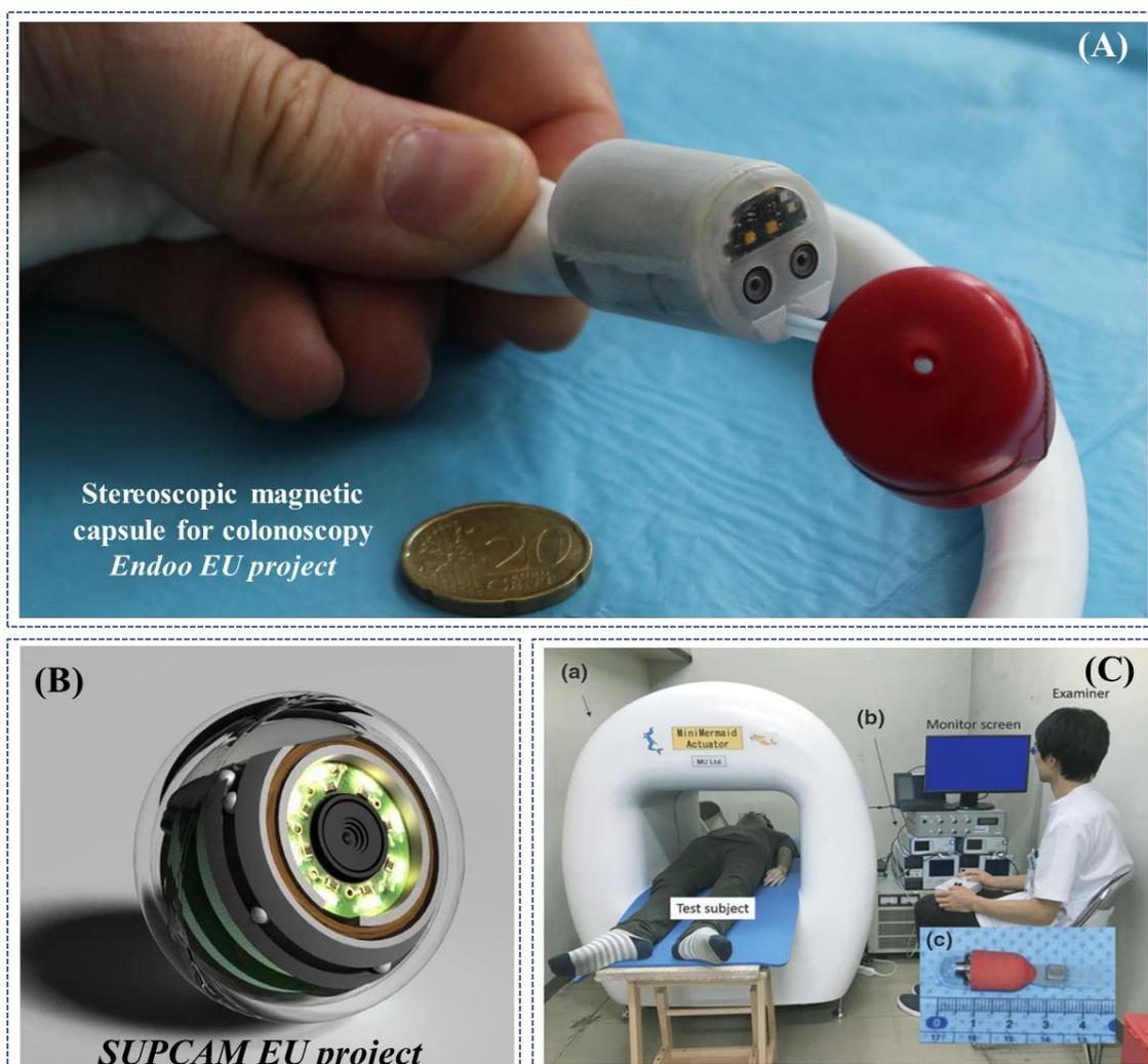
**Figure 6.** Examples of research-oriented innovative robotic colonoscopes and devices with magnetic or electromagnetic actuations: (A) Endoo EU project capsule (Courtesy of the Endoo consortium); (B) SUPCAM EU project spherical magnetic capsule for colonoscopy (Courtesy of Dr. Alessandro Tozzi); (C) modified PillCam™ SB2 with a silicone fin for magnetic locomotion through external electromagnetic fields, developed by Nouda et al. [128].
