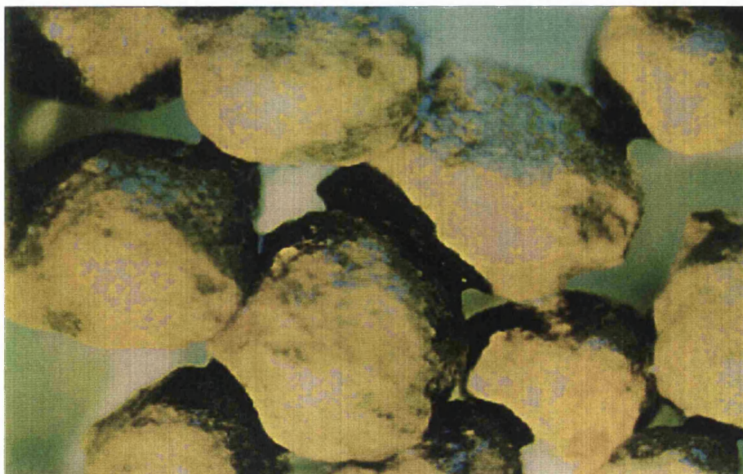
Figure 8.18: 2.8-5.6mm Media Particles From Middle of Filter Bed (HLR 1)
