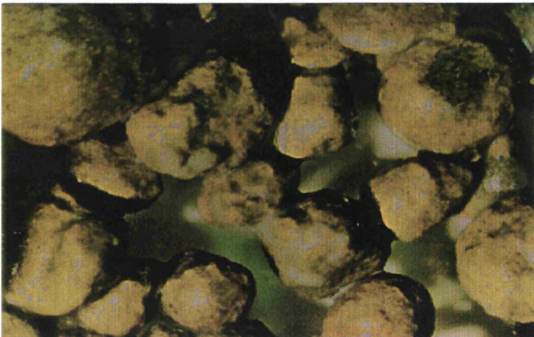
Figure 7.22: 2-4mm Media Particles From Middle of Filter Bed (HLR 4)
