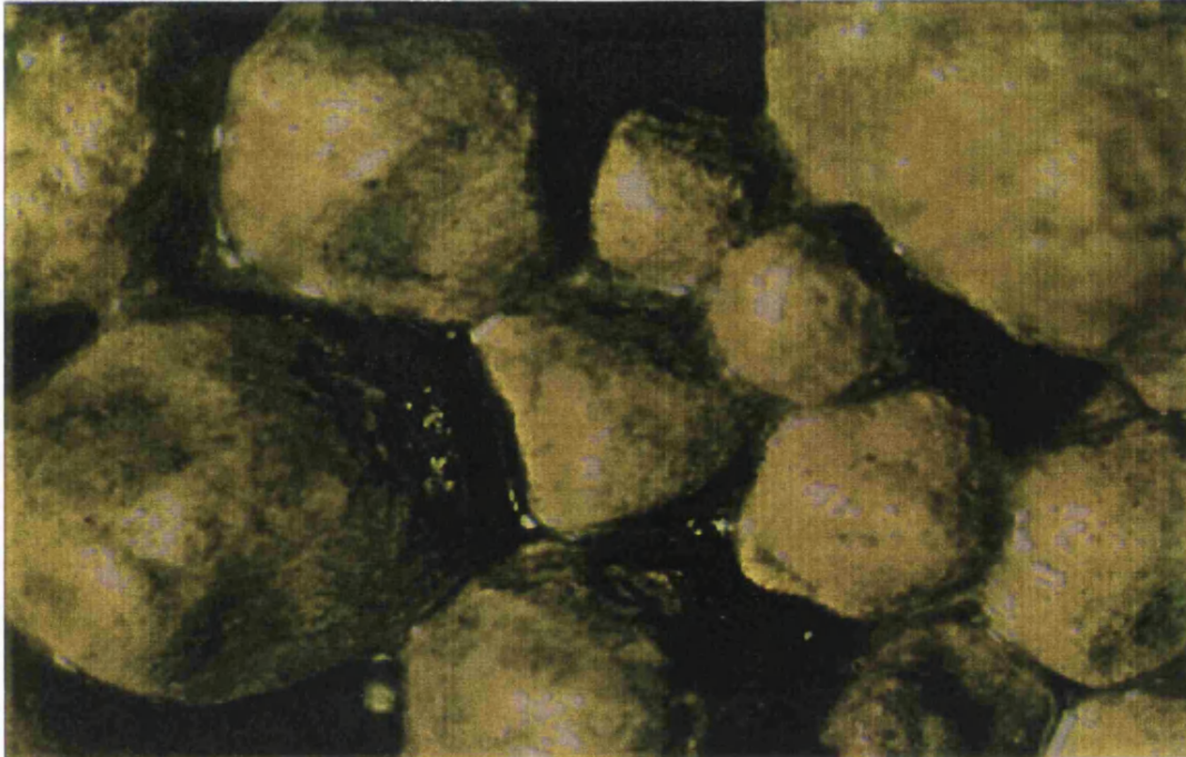
Figure 8.19: 2.8-5.6mm Media Particles From Middle of Filter Bed (HLR 4)
