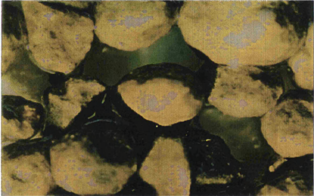
Figure 7.21: 2-4mm Media Particles From Middle of Filter Bed (HLR 1)
