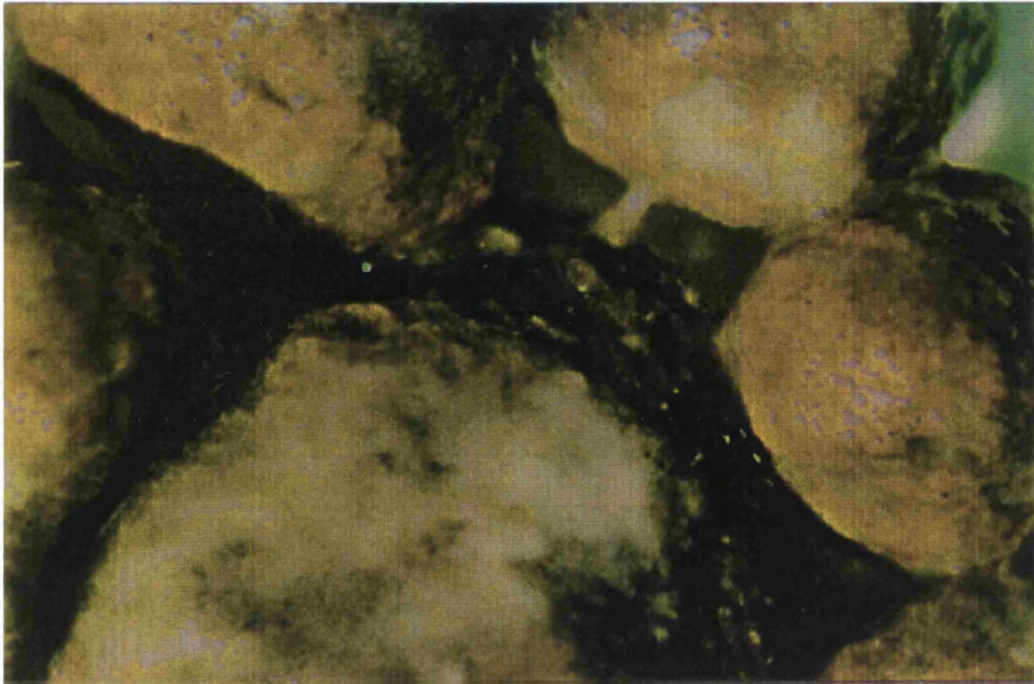
Figure 9.19: 4-8mm Media Particles From Middle of Filter Bed (HLR 4)
