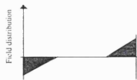
Fig 2.17 Field distribution in an MSM diode
