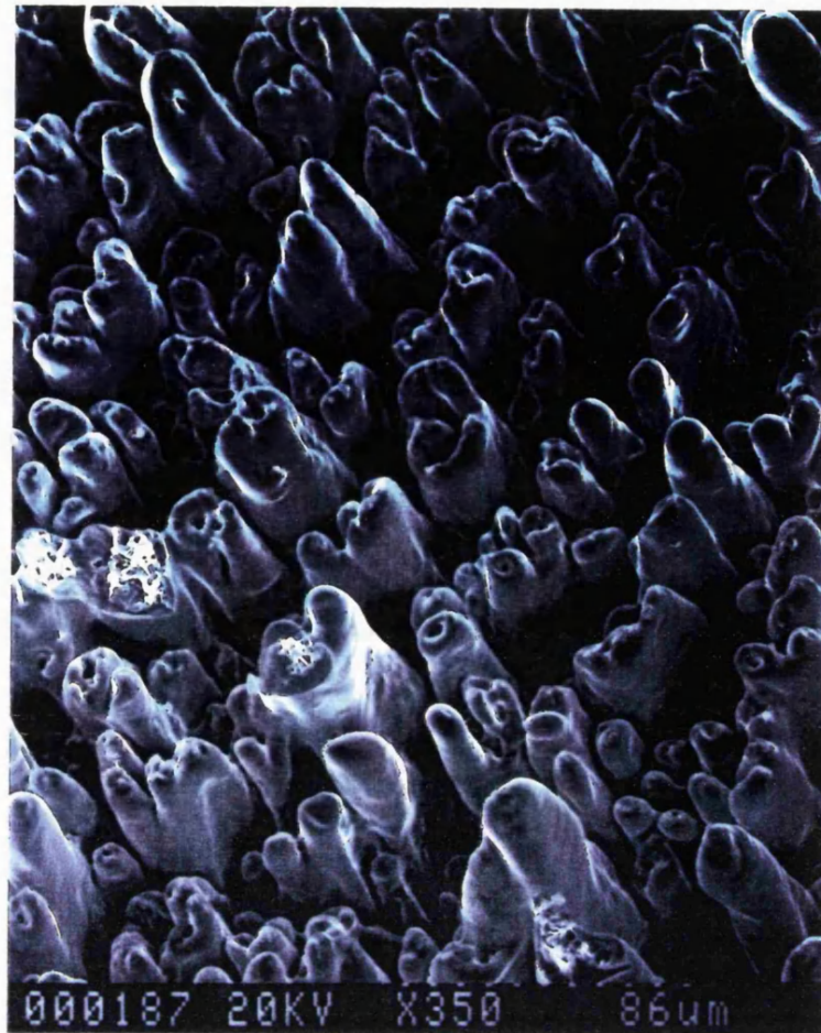
Figure 3.4- SEM photograph of a BiPbSrCaCuO (2212) pellet after irradiation with 1000 pulses of 1.6\text{J}/\text{cm}^2 .
