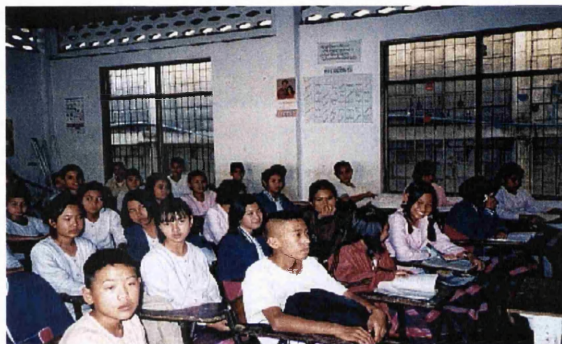
Figure A12.1 Condition of windows; good windows (no broken frames, the lower border of windows is high above floor [at least 1 metre])
