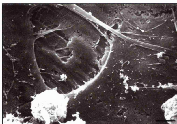
Figure 3.17 SEM showing multilayering of U2-OS cells on polished Zr at 10 days of culture. No collagen fibres could be identified. Round shaped shrunken cells can be seen on top of the cell layer. Bar denotes 2 \mu\text{m} .
