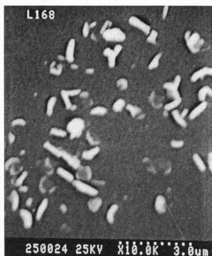
Figure 5.21 SEM image of the film deposited from the reaction of [\text{Me}_3\text{SnS}_2\text{CNEt}_2] with hydrogen sulfide at 450 °C.
